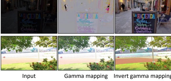
Figure 3. Outputs of the gamma and invert gamma mappings. The output of the latter is visibly better than that of the former.
