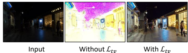
Figure 10. The influence of the total variation loss. Without the loss, the gamma values of neighboring regions are not so smooth, thus breaking down the image structure.
